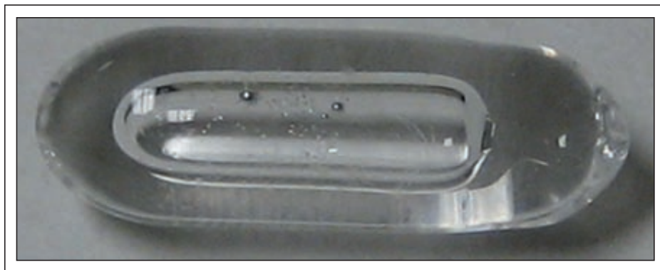
Fig. 3: The electrode-less bulb.
